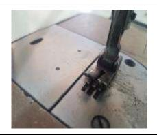
It was noted during factory tour that needle guard were missing on 25% sewing machines.
